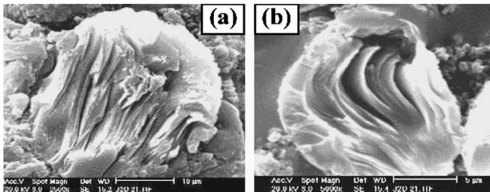
Figure 4 Complicated structures of MCMB2 detected by SEM.
