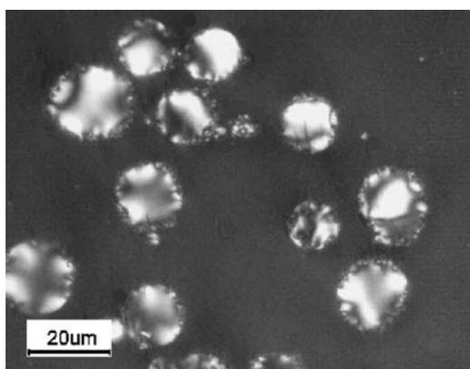
Figure 3 Optical characteristics of MCMB2, which are contained in MP2, under polarized light microscope.
