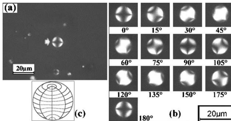
Figure 1 Optical characteristics of MCMB1, which are still in MP1, under polarized light: (a) a typical micrograph, (b) regular extinction contour changes of the sphere pointed out in a by the arrow when rotating the stage per 15° anticlockwise, and (c) model structure of Brooks-Taylor-type MCMB.
